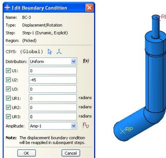
Fig 7: shows the boundary condition applied for the plunger and the billet
