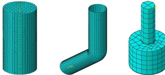
Fig 6: shows the meshed geometry of plunger billet and die
