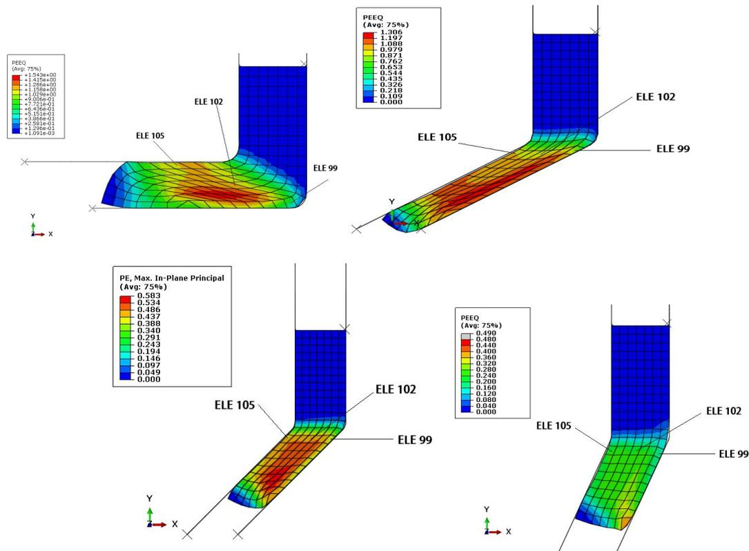
**Fig 8:** Shows that the shear stresses along the curvature for all channel angles
