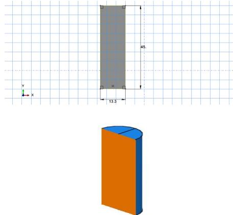
*Fig 3: Shows the billet part both 2D and 3D*
