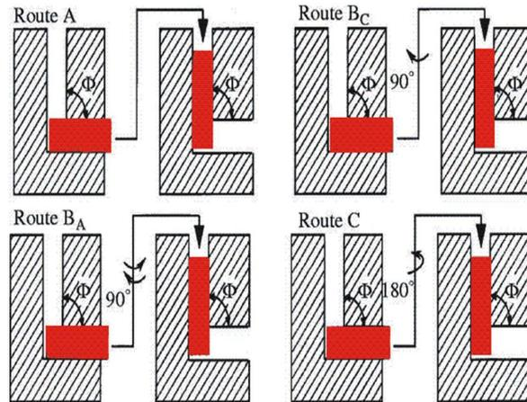
*Fig 2: Shows the four fundamental processing routes used in ECAP process*
