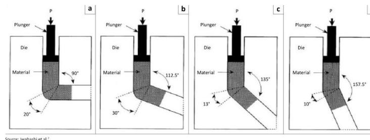
*Figure 1: Shows various channel angles of ECAP*
